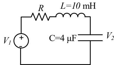
a. Determine the transfer function of the system in terms of  $R$  ( $G(s) = V_2(s)/V_1(s)$ ).
